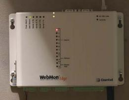
The WebMon Edge monitors discrete inputs, network devices, environmental conditions with built-in sensors, its own power supply, and all types of external conditions through a Modbus interface. The Edge can also monitor its own location with a GPS module, useful in vehicles or other portable installations.
