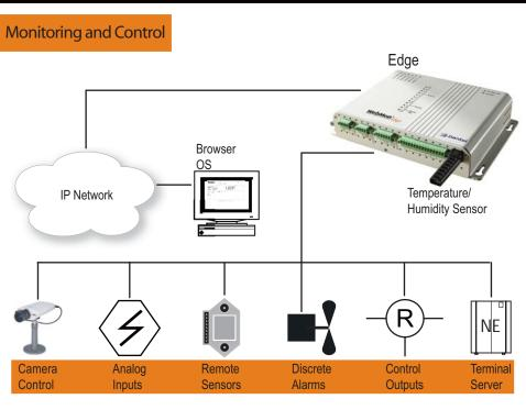
The WebMon Edge is a fully integrated remote monitoring and surveillance appliance combines telemetric, transport and security capabilities into a single platform, for integrated operation in any environment. With the Edge, you will sense dangerous events or conditions long before adversely affect your critical infrastructure.
