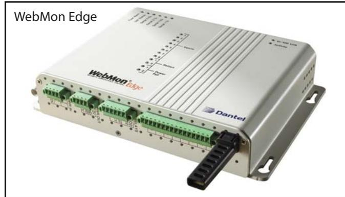
Dantel's WebMon Edge is a remote surveillance and management network appliance. The Edge monitors virtually any type of sensory input with its expanded sensor capabilities, providing remote alarm monitoring, visual verification, and remote office control.
